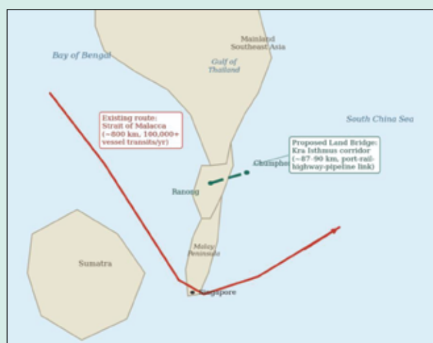
Figure 1. Schematic comparison of the existing Strait of Malacca route and the proposed Kra Isthmus Land Bridge corridor. Illustration prepared for this article.
